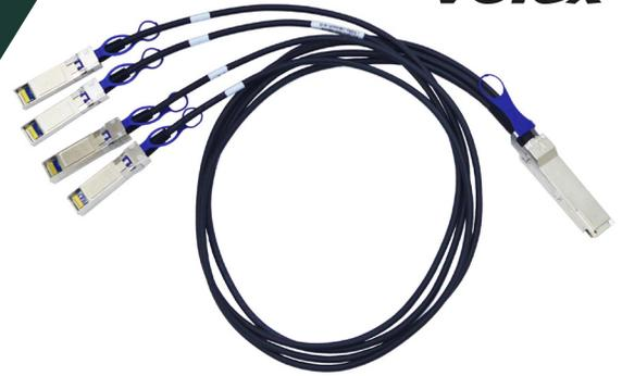
Volex's QSFP+ Passive Breakout Direct Attach Cables feature 4 transmitting and 4 receiving channels at 10Gbps data rate per channel. 40Gbps (QSFP+) to 4x 10Gbps (4x SFP+) breakout configurations is supported. The cable assemblies meet 40Gbps Ethernet (IEEE 802.3ba) standard with substantial signal integrity margin providing high performance and bandwidth interconnect solutions for high density applications.
